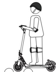
⚠ Keep your speed between 5-10 km/h when you ride through speed bumps, elevator door stills, bumpy roads or other uneven surfaces. Slightly bend your knee to better adjust mentioned surfaces.
