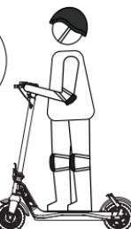
2.Step on the deck with one foot, and slowly kicks off the other on the ground. When the scooter starts to coast, put both feet on the deck and press the accelerator. Note: The accelerator initiates once the coasting speed exceeds 5 km/h.
